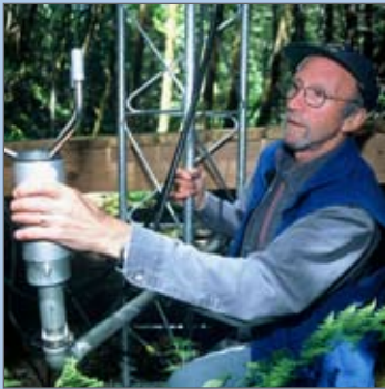
Michael Unsworth installs an instrument to measure gases given off by trees.
