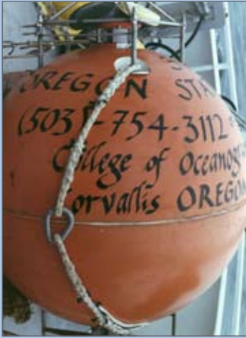
Acoustic Doppler Profiler ready for deployment during Coastal Transition Zone, with written instructions for return of the buoy, in case the mooring is accidentally destroyed.
