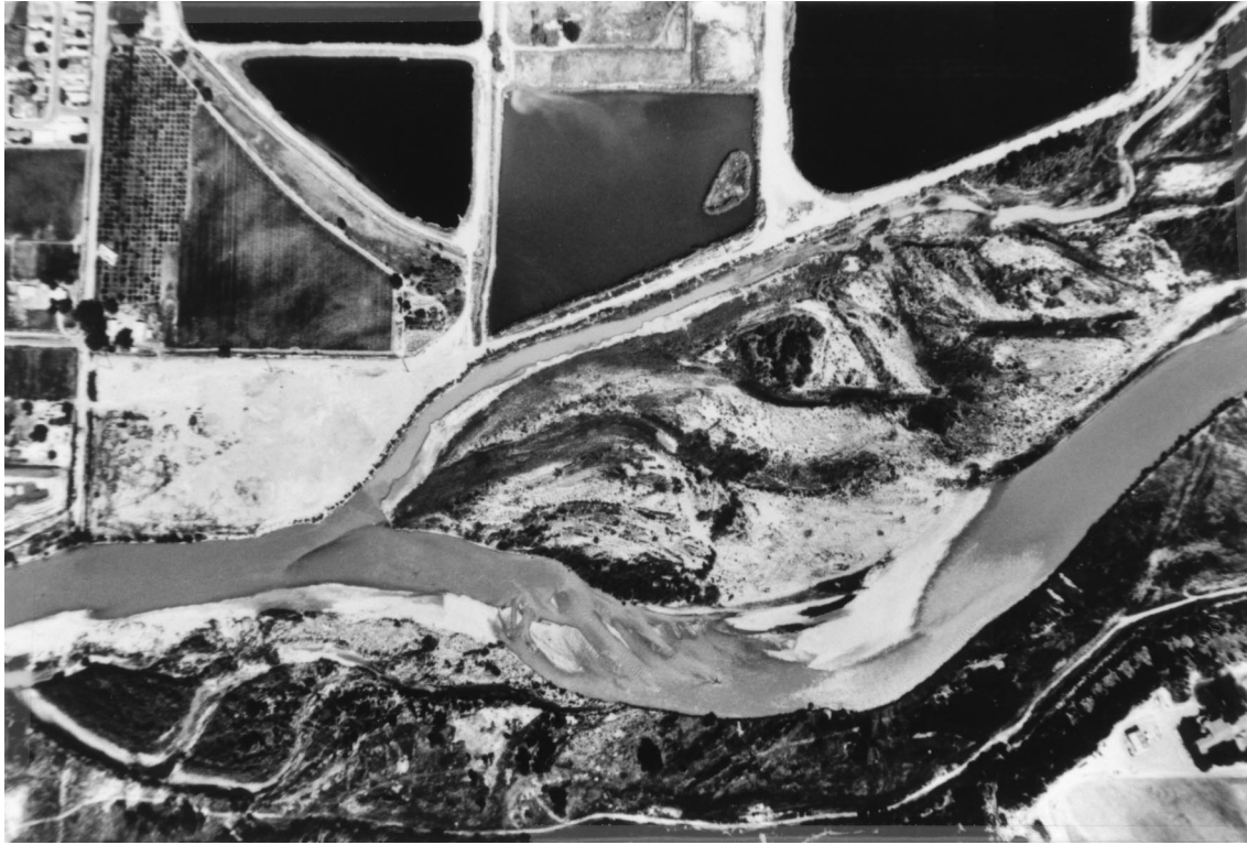
Figure 1. Aerial photograph of a segment of the Colorado River in the 15-mile reach. This photograph shows a dissected gravel bar, portions of two runs, a stable island, and a relatively long backwater. The trapezoidal pond with the small island is 250 m across. Flow is from right to left.
